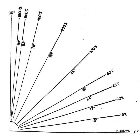
Expressing slope as a percentage permits easy comparison of the relationship of the vertical (rise) to the horizontal (run). For example, a 30% slope will rise 30 m vertically over a horizontal distance of 100 m.
